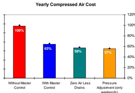
After the initial audit a master control with an integrated online monitoring system can provide all data necessary to verify improvement projects.
